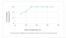
BC-30 Vet utilizes a temperature control system to stabilize reaction temperature, eliminating the clogging problems and resulting in accurate test results that come from operating in cold environ-
